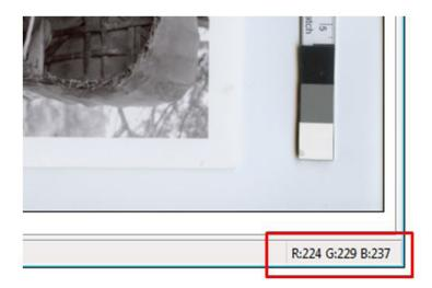
**3.3.4** The readings on the black end of the greyscale patch should be **within 15** of the following figures:
